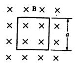
A square loop of wire of resistance R and side a is oriented with its plane perpendicular to a magnetic field B, as shown above. What must be the rate of change of the magnetic field in order to produce a current I in the loop?
